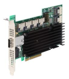
up to 24 drives inside the server via direct connection or passive backplane. Using the external SAS ports, multiple JBODs can be connected to a server, providing a scalable and affordable solution for growing storage requirements. The RS2SG244 supports data transfer rates of up to 6Gb/s per port, and brings new features and improved performance regardless of whether the storage solution utilizes 3Gb/s or 6Gb/s SAS or SATA drives.
